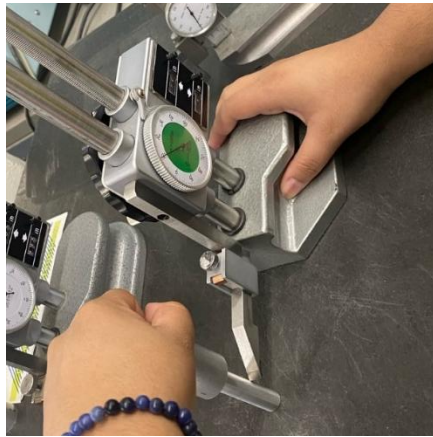
Figure 17. Marking where keyway will end
