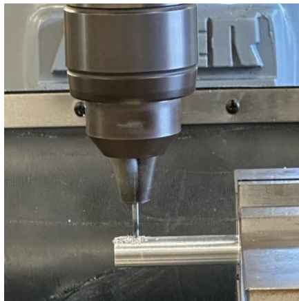
Figure 18. End milling keyway into pinion shaft
