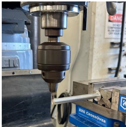
Figure 23. Adding keyway on ring gear side shaft
