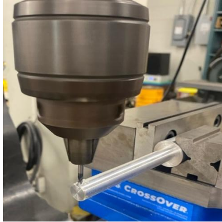
Figure 21. Adding keyway on spider gear side shaft
