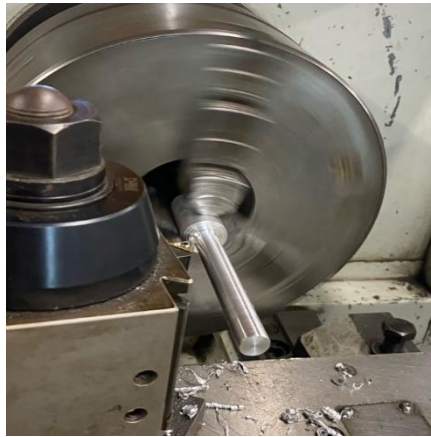
Figure 19. Reducing diameter of spider gear side shaft
