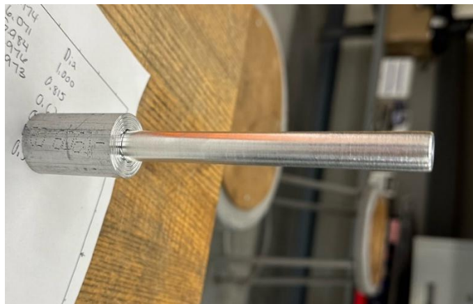
Figure 24. Ring gear side shaft
