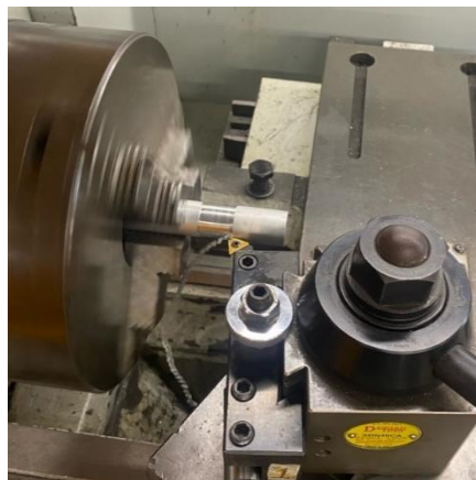
Figure 15. Reducing diameter of pinion shaft
