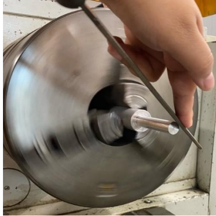
Figure 16. Adding chamfer to pinion shaft
