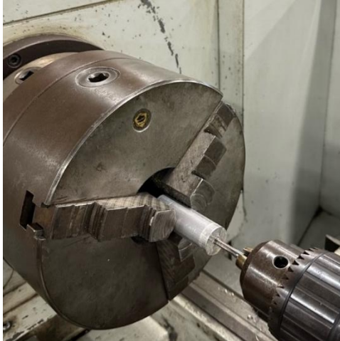
Figure 11. Threading spider gear shaft hole
