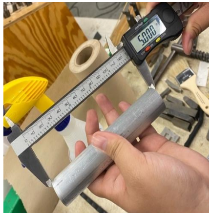
Figure 14. Final length of pinion shaft
