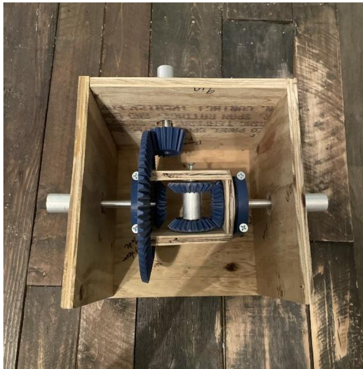
Figure 30. Top-down View of Assembled Differential
