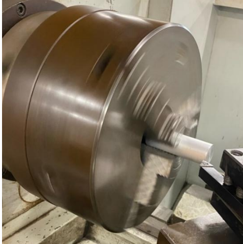
Figure 8. Reducing length of spider gear shaft
