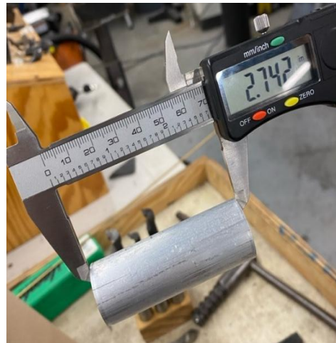
Figure 9. Final length of spider gear shaft
