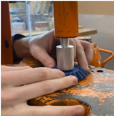
Figure 4. Press fitting the bearings into the gears
