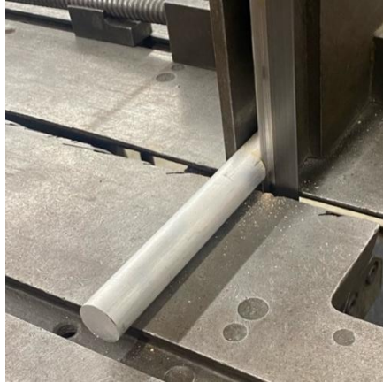
Figure 22. Cutting shaft using bandsaw
