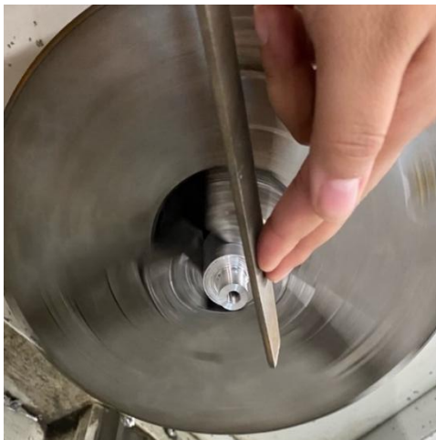
Figure 13. Adding chamfer to reduced diameter
