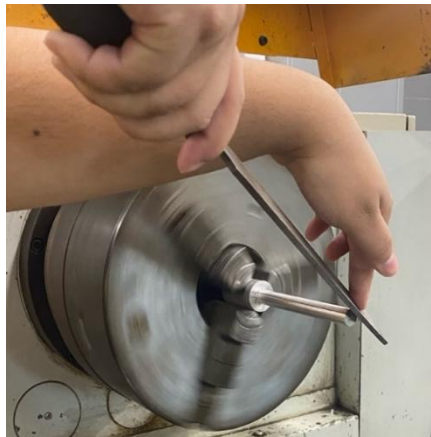
Figure 20. Adding chamfer to spider gear side shaft
