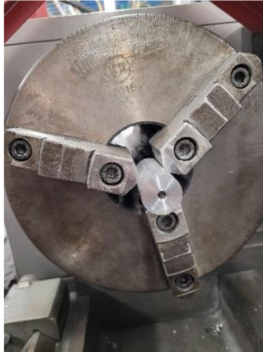
Figure 6. The shaft on the Jet lathe after the center hole has been drilled
