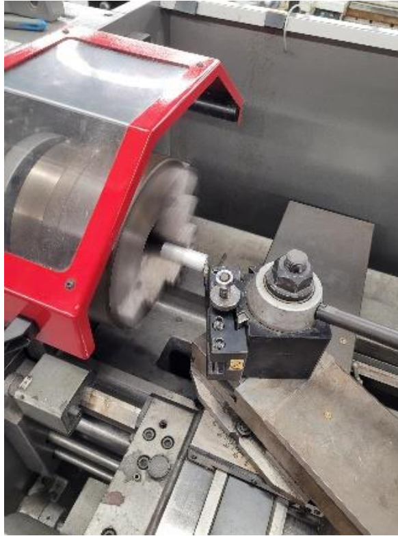
Figure 5. The shaft on the Jet lathe being turned to 2.502 inches
