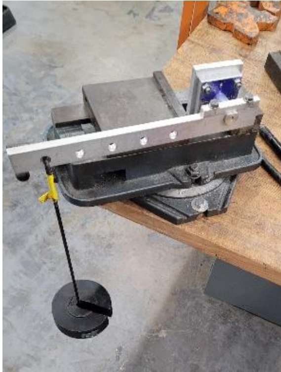
Figure 8. The completed assembly enduring the 10 foot-pounds of force
