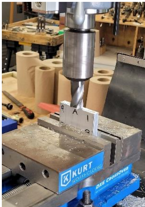
Figure 2. The plate being face milled on the Acer milling machine
